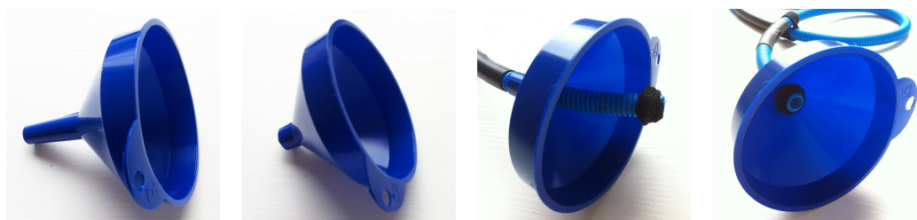
Figure F.3: Turning a plastic funnel into a bell.
